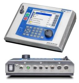
The controller includes two print head ports for up to 512 total nozzles, Ethernet, serial, and USB ports, and a freely programmable digital I/O port.
