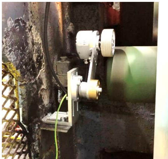
Encoder with wheel and spring-loaded bracket
