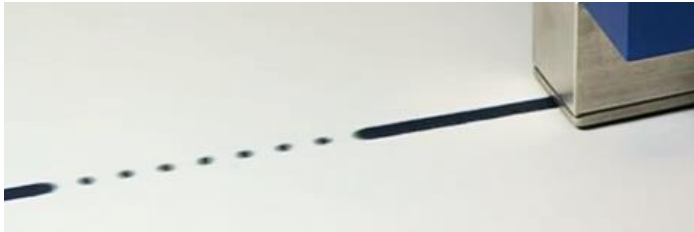
Dot and Line Marking with EDS + EDC Controller
