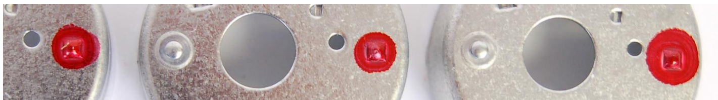
Close-up view of three excellent quality marks from our lab. Note that the mark is a splatter shape.
