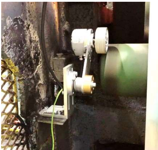
Encoder with wheel and spring-loaded bracket
