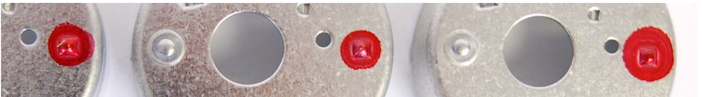
Close-up view of three excellent quality marks from our lab. Note that the mark is a splatter shape.
