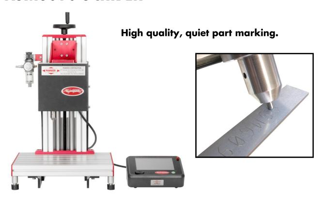
The ASM6090 Scriber is a quiet and fast system for marking metals and plastics. It offers a generous marking window in a compact marking head. The Carboloy marking pin extends onto the material being marked and then the pin is moved to create marks consisting of solid lines for high-quality engraving.
