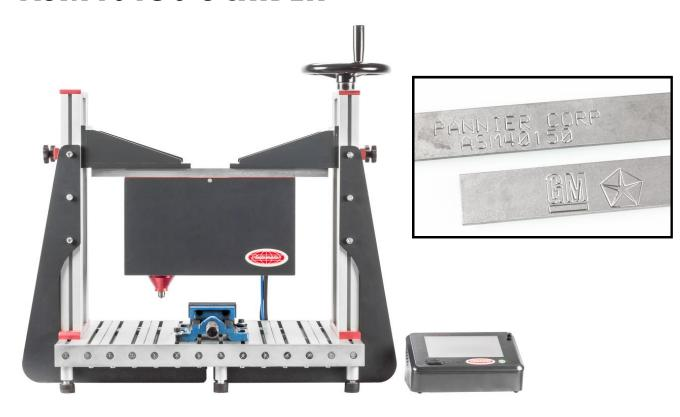
The ASM40150 Scriber is a heavy-duty, yet quiet system for marking metals and plastics. Its 40mm x 150mm marking window accommodates marking jobs requiring one or more long lines of text and logos. The Carboloy marking pin extends onto the material being marked and then the pin is moved to create marks consisting of solid lines for high-quality engraving.
