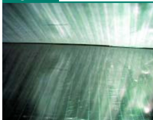
View of a highly reflective tinplate surface, differentially marked on the heavy-coated side.
