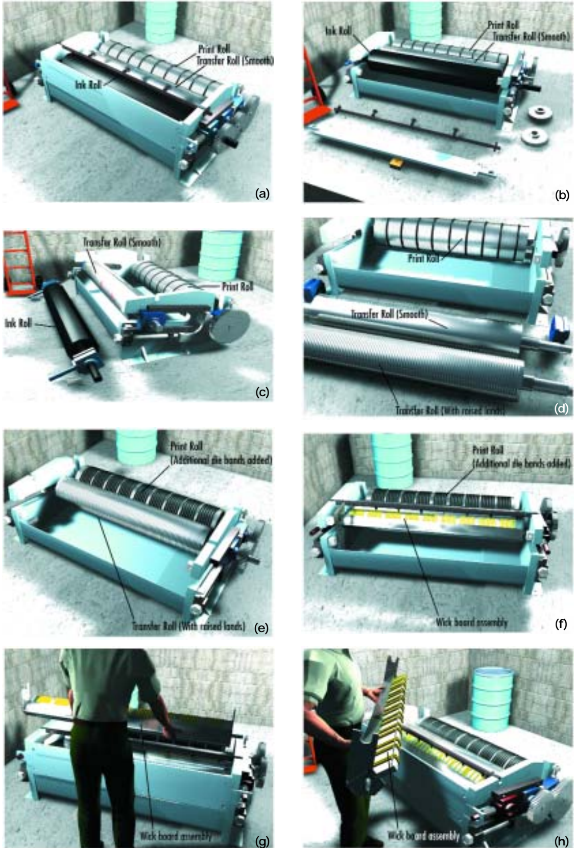
Steps involved in replacing the pickup roll with a wick board assembly: (a) before conversion; (b) pickup and transfer rolls prepared for removal; (c) pickup and transfer rolls being removed; (d) new transfer roll with raised lands; (e) new transfer roll installed; (f) wick board assembly installed; (g) view showing easy removal of wick board; and (h) view showing the use of multiple wick board patterns.
