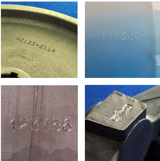
Mark part numbers, date codes, and logos on materials such as metal, plastic, wood, and even paperboard.
